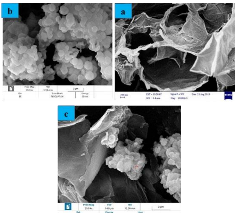
Fig. 2. The FE-SEM images of the as-synthesized (a) rGO, (b) Cu-L complex (c) Cu-L/rGO.
