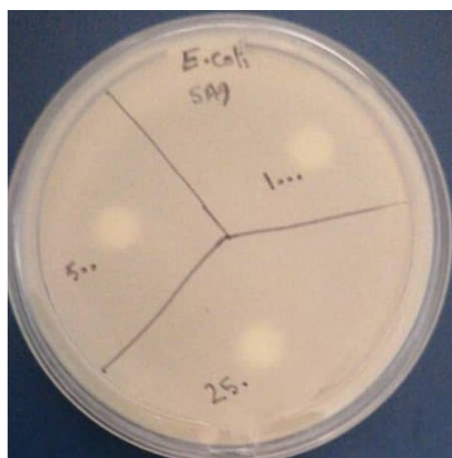
Fig. 6. Zone of inhibition test for bismuth sample against E. coli using standard antibiogram disks. All tested concentrations (1000, 500, 250 \mu\text{g/ml} ) resulted in zero inhibition.
