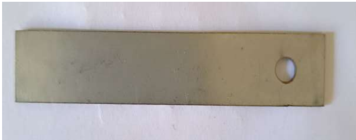
Fig. 1. The image of the used C1018 alloy sample 8.7 cm × 1.4 cm × 0.1 cm.
